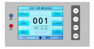
Light panel schematic diagram is shown in Picture. Above title display light name. Below is the status bar, show current light signal, lamp status, fault (When there is a fault message not viewed, display "ERR", no is display "NOR"). etc.
