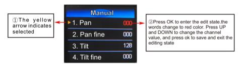
This interface is to control current fixture, meanwhile enter master status (Not receiving DMX signal, but sending to slave fixtures.)
